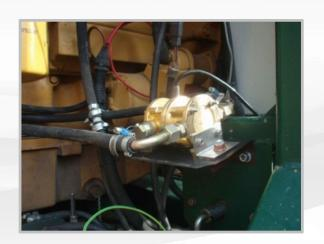
Type of use: CAT excavator 904 Type of fuel meter: DFM 8 D
