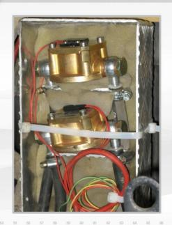
Type of use: CAT bulldozer 242B Type of fuel meter: VZO 8 OEM
