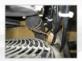
Type of use: CAT bulldozer 428E Type of fuel meter: DFM 8 D
