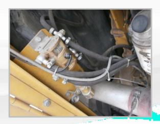
Type of use: CAT bulldozer 988H Type of fuel meter: DFM 8 ECO
