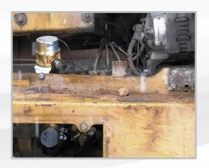
Type of use: CAT bulldozer D6R Type of fuel meter: VZP 8
