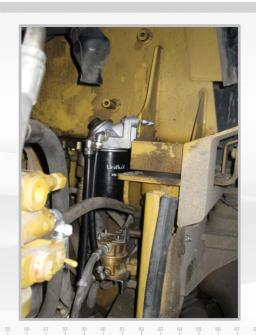
Type of use: CAT bulldozer 938G Type of fuel meter: DFM 8 D
